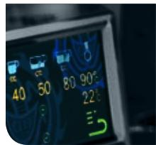
Each intelligent display controls the thermoregulation of each group, the adjusting of the coffee dose and the infusion time, all in real time.
